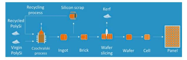
**Step 1** - PolySi: The raw material used to produce the cells is a high purity silicon called "Solar grade silicon" or "PolySi".
