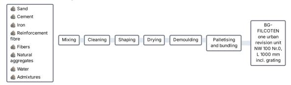
Drainage channels out of concret - FILCOTEN® HPC (High Performance Concrete) - for vehicular and pedestrian areas according to standard EN 1433
